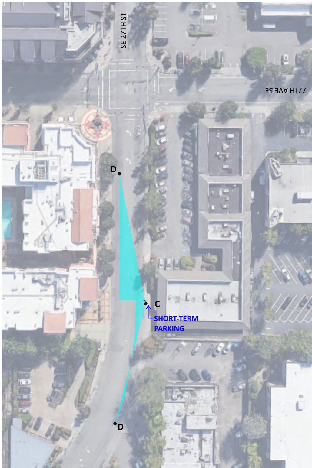
POINT C - DRIVER'S EYE 14.5-FT OFFSET FROM EDGE OF TRAVEL-WAY (SE 27TH ST), CURVED TO SHOW APPROXIMATELY WHERE THE DRIVER'S EYE IS FOR THE CAR IN SHORT-TERM PARKING SPACE POINT D - INTERSECTION, OR ENTERING, SIGHT DISTANCE (335-FT) ALONG TRAVEL-WAY; 30 MPH DESIGN SPEED
